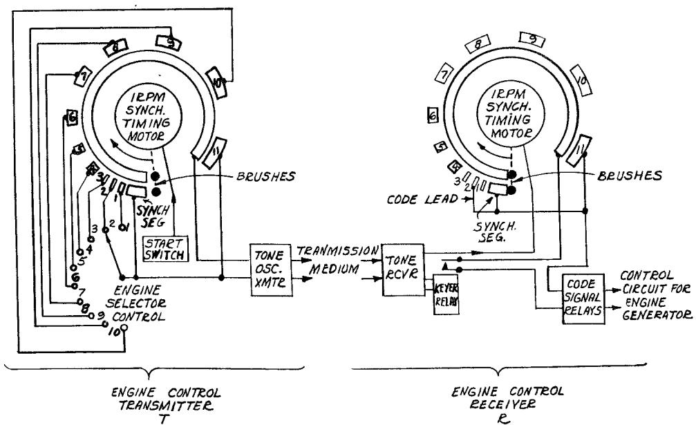
Fig. 2 - Simplified diagram of engine generator remote control scheme.
