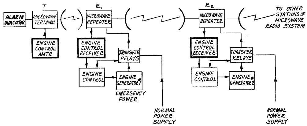
Fig. 1 - Block diagram of typical system using remote engine generator control. Units described in this paper shown in heavy outline.
